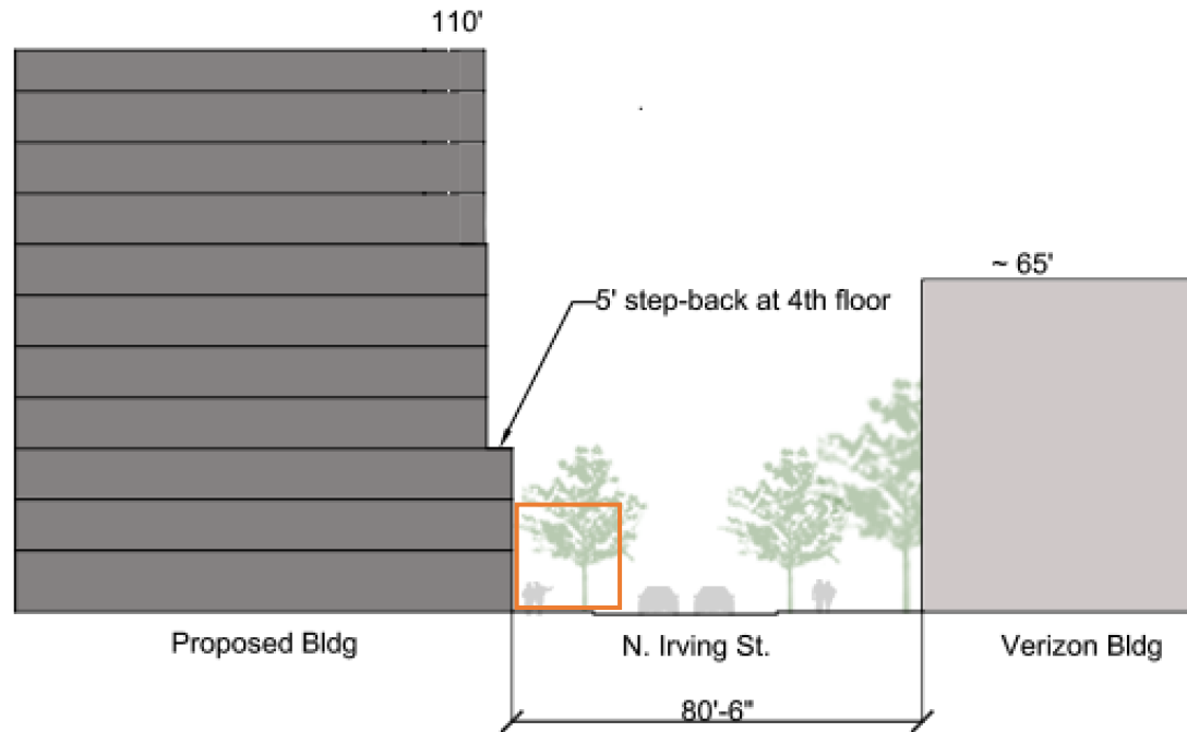
Staff Alternative 1 Section Looking North
