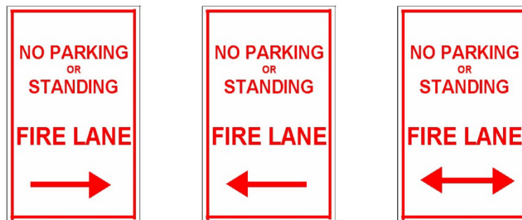
Figure 503.3.2 Fire lane signs
