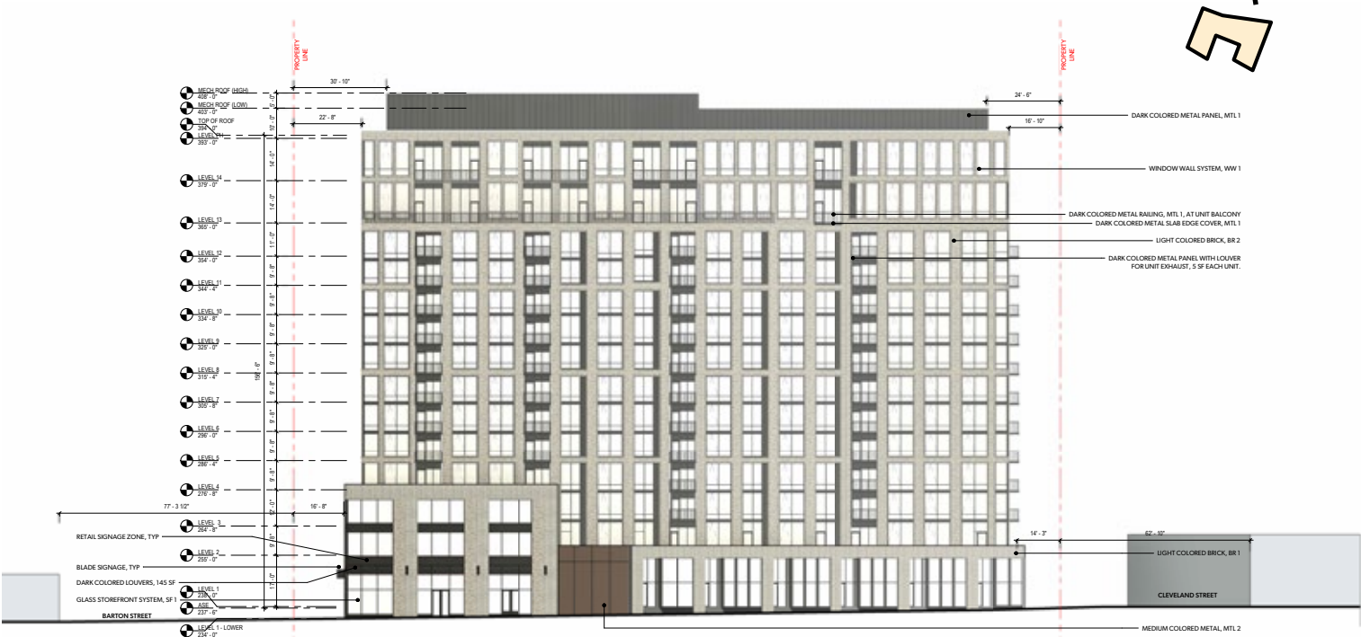
BUILDING ELEVATION - WILSON BLVD
