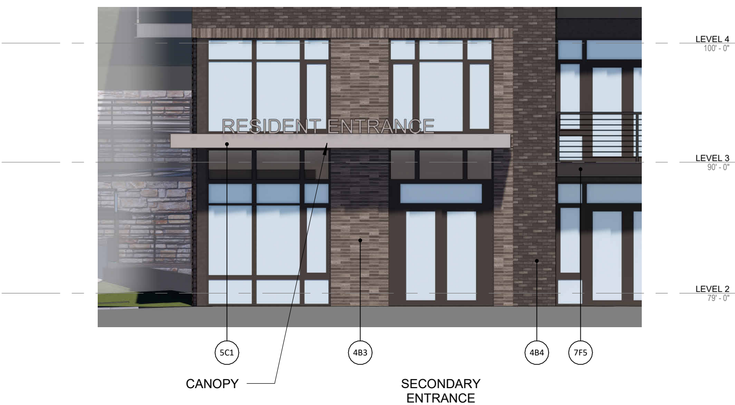
5 --- BLDG E - LEVEL 1 ENTRANCE ENLARGED ELEVATION
