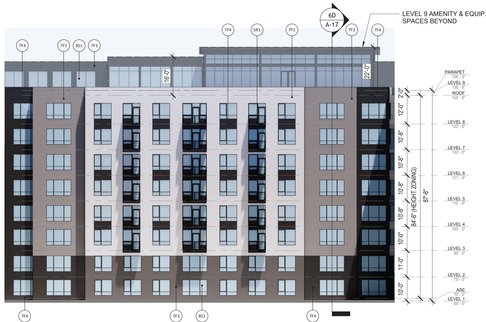
5A BUILDING E - COURTYARD WEST ELEVATION
