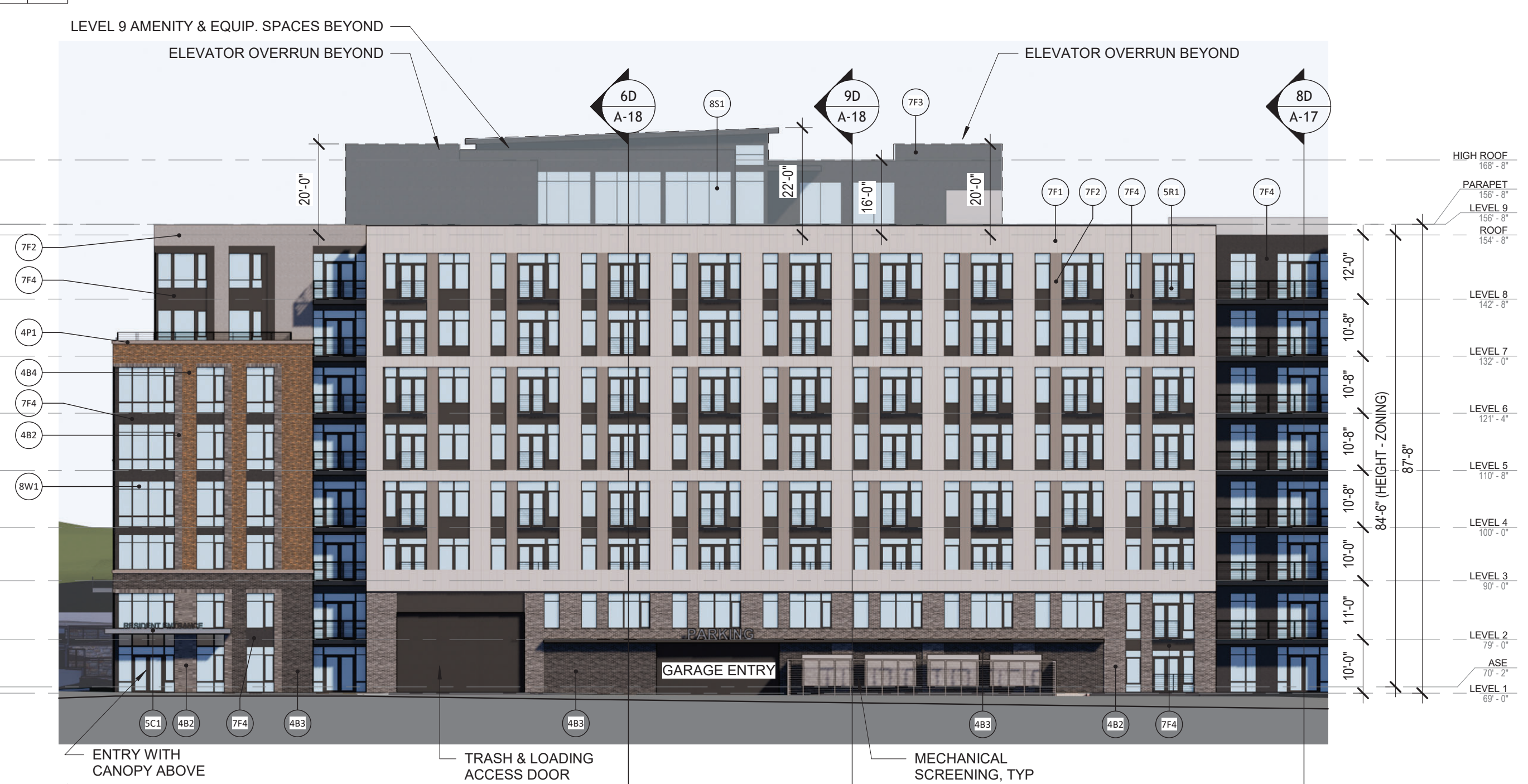
7A BUILDING E - SOUTH ELEVATION 1 A-02 A-21 1" = 20'-0"
