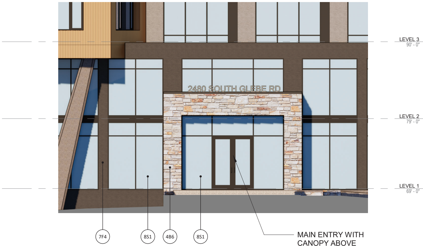
4 --- BLDG E - LEVEL 2 ENTRANCE ENLARGED ELEVATION
