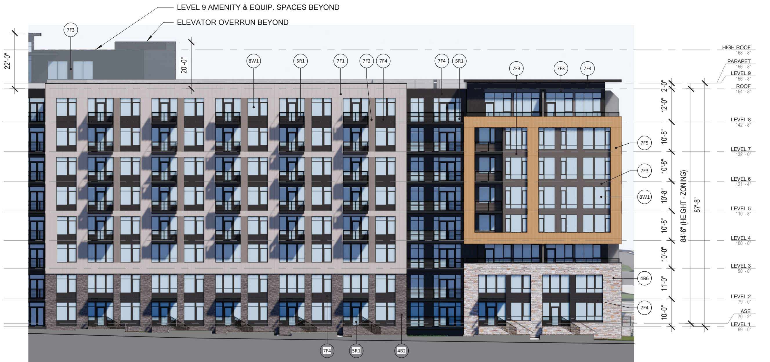
7F BUILDING E - SOUTH ELEVATION 2 A-02 A-21 1" = 20'-0"
