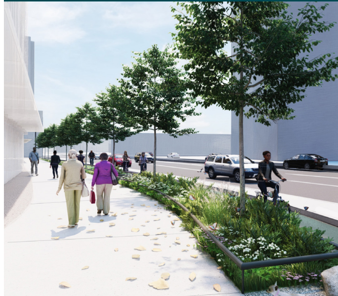
TYPICAL SIDEWALK (MIN. 10' CLEAR)
