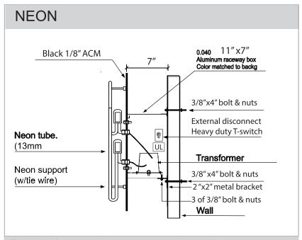
This sign is intended to be installed in accordance with the requirements Article 600 of the National Electrical Code and/or other applicable local c this includes proper grounding and bonding of the sign
