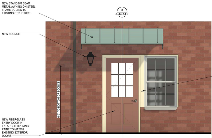
2 ENLARGED ELEVATION - ACCESSIBLE ENTRANCE
