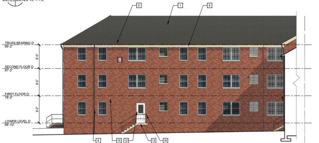
3 BUILDING 41 ELEVATION G A-41-2.0 | A-41-4.4 1/8" = 1'-0"
