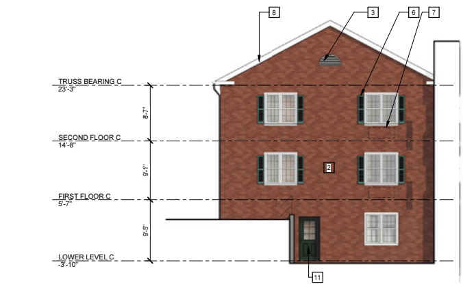
3 BLDG 5 ELEVATION C - PARTIAL NORTH A-5-2.0 | A-5-4.1 1/8" = 1'-0"
