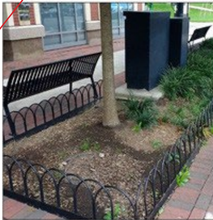
examples of inappropriate mechanical equipment configurations visible from the STREET
