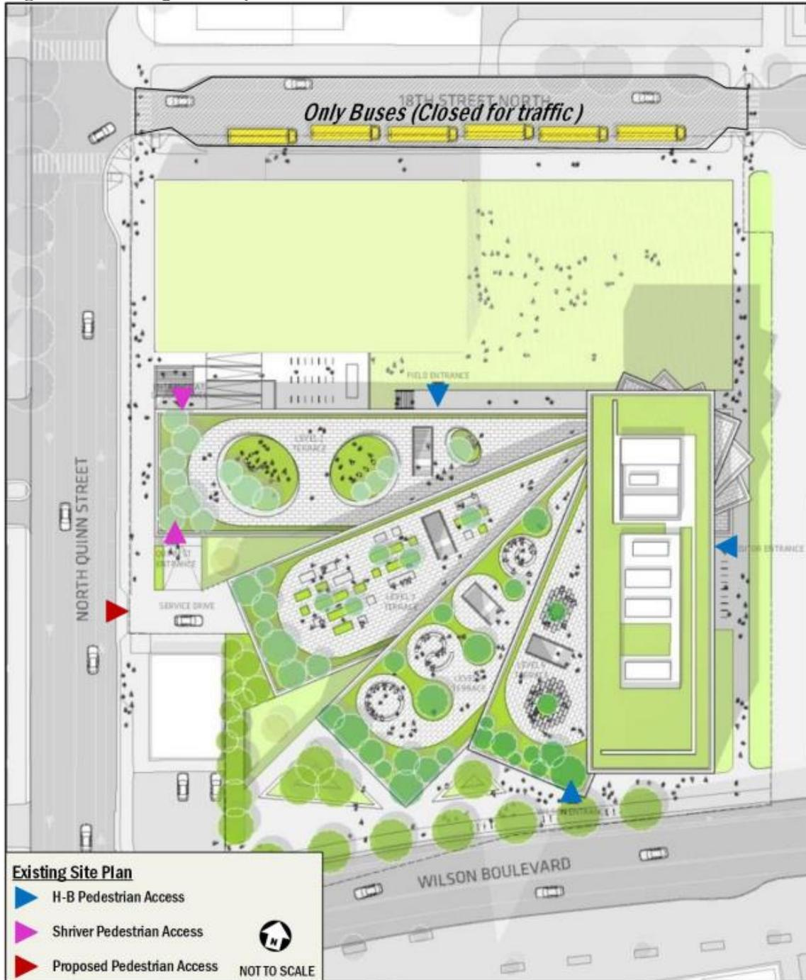
**Proposed Development:** The following figure depicts the proposed below-grade parking structure with 61 spaces, entrance/exit on 18th Street North, a covered entrance to the Shriver Program, bike parking, storage for APS equipment, and a lighted synthetic turf field above the garage with amphitheater seating in the northwest corner where the field tilts upwards.
