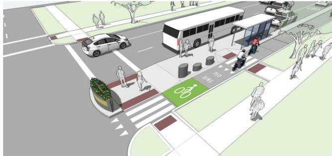
and bikes at bus stops located between transit/traffic lanes and bicycle lanes, the floating bus stop island provides a safe area where transit passengers can board and alight transit.
