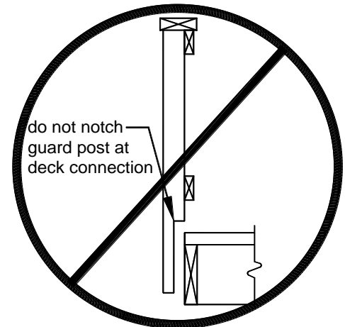
FIGURE 27: PROHIBITED NOTCHING AT GUARD POSTS
